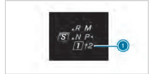
▶ If gearshift recommendation message ① is shown on the multifunction display, shift to the recommended gear.
