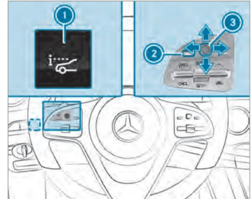
The on-board computer is operated using left-hand Touch Control ③ and left-hand back/home button ②.
