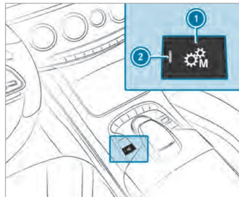
▶ **To activate/deactivate:** press button ①. If indicator lamp ② is lit, manual gearshifting is activated. The current gear is displayed in the multifunction display.
