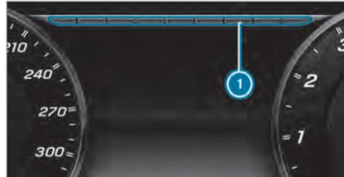
If the engine speed is too high or too low, you cannot change gear using the steering wheel gearshift paddles. In this case, segments ① light up red.
