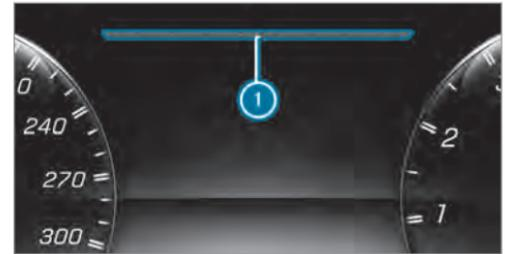
If the engine speed is too high or too low, you cannot change gear using the steering wheel gearshift paddles. In this case, segments ① light up red.
