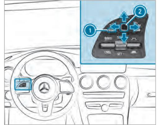
The on-board computer is operated using left-hand Touch Control **②** and left-hand back/home button **①**.
